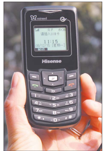
Qualcomm's mirasol display, which mimics the way light reflects off the scales of butterfly wings, can be viewed in direct sunlight as well as very dark environments.
